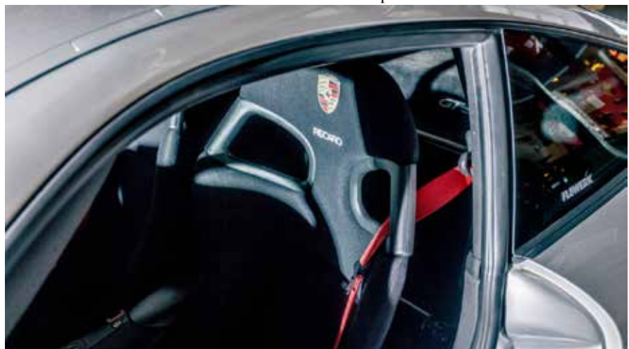
A look inside: The 911 GT3 (996) has a bucket seat covered with heat and flame-resistant Nomex, a permanently installed roll cage and six-point seat belts.
