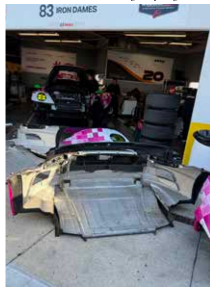
Here are the front and rear panels, they can be change in about 2-3 minutes during a pit stop if no structure damage has occurred
