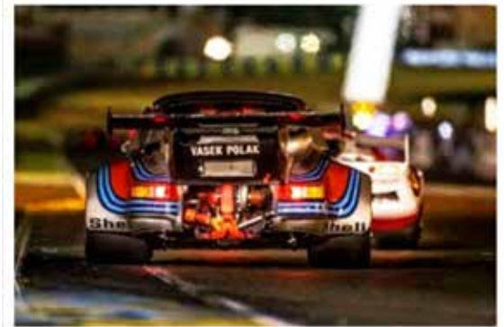
Glowing-red turbocharger on a Porsche racecar shows the extreme temperatures that the turbocharger is subjected to
