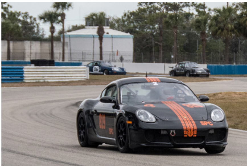
Above: Keith Fritze rockin' through T11 at Sebring. Interesting photo in that you can really see how loaded the right rear tire is as compared to the left front. Gives you a good idea why you get understeer in a turn like this. Slow exit from T10 and then a sweeper in the other direction.
