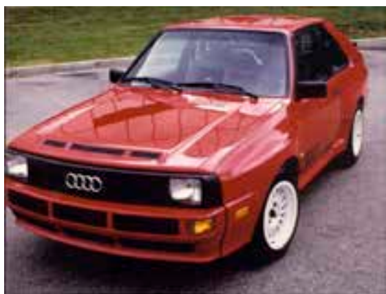
1984 Audi Sport Quattro: 2.2 liter, 5 cylinder, 485 hp 4WD (155 mph top speed)
