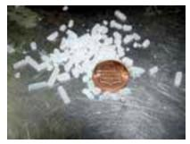
"The machine is fairly simple", he said, "it's a big air compressor which generates very dry, pressurized air, then uses the pressure and a venturi to add the CO2 pellets to the stream of compressed air through a hose. Before
