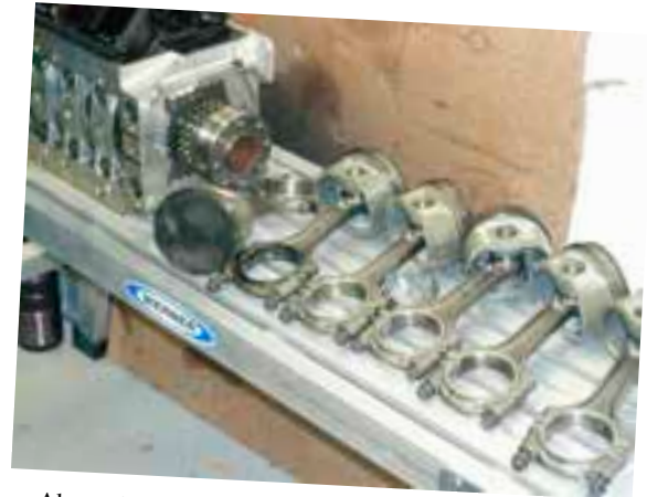
Above: The cradle and the pistons (note the scorching on #4 arm)
