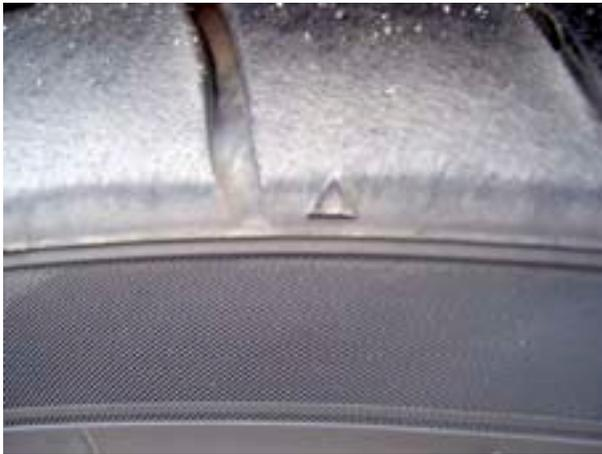
the track again gives us the optimal patch, as seen below where the edge of the wear is right to the tip of the marker.
