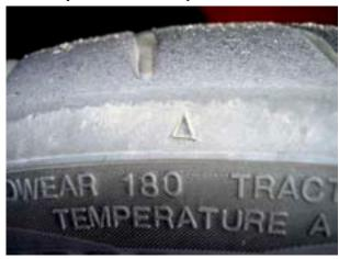
Most modern high-speed rated tires have special markers to show us the optimal tire patch.
