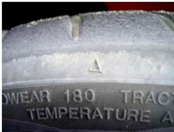
Most modern high-speed rated tires have special markers to show us the optimal tire patch.
