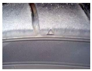
the track again gives us the optimal patch, as seen below where the edge of the wear is right to the tip of the marker. Also, always keep in mind that you should never inflate beyond the tire's maximum pressure, stamped on its sidewall.
