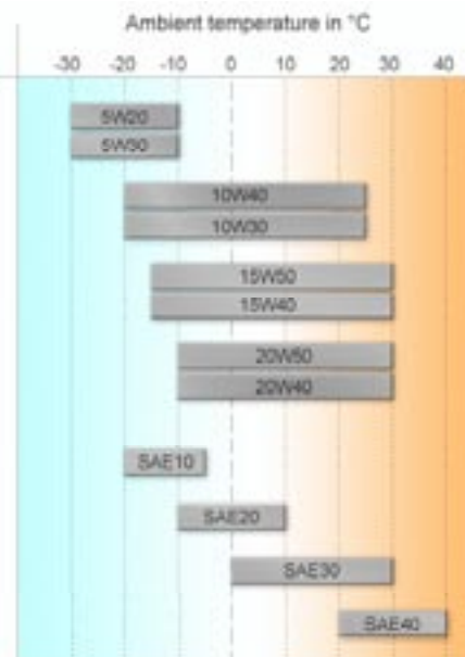
Figure 2 – Viscosity Service Ranges
