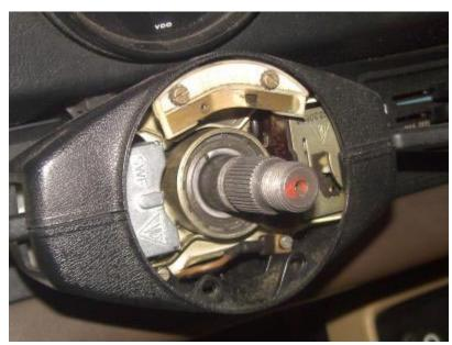
replace the failed plastic piece with a new plastic sleeve. Unfortunately these aftermarket sleeves are not easily installed as advertised and cost about \$15.00 plus shipping. They are made of plastic, similar to the failed piece that started the whole process. Instead of a temporary fix, here is a permanent solution. Install a steel sleeve instead. A sleeve borrowed from a 928 of course. The sleeve (part #928.347.739.02) is a perfect fit into the 911 column. The cost is only \$6.27.
