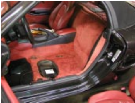
Figure #2: When the drain holes become clogged, the excess water will saturate this back carpet piece until a pool of water collects under the seat (and over the control unit).
