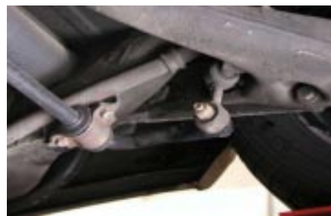
Figure 2: Type-2 sway bar (21mm) with stock mounting on a 911SC
