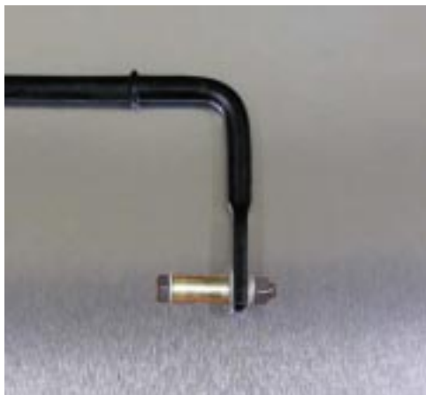
Figure 4: A type-2 sway bar modified with the kit shown in figure #5; It now can be used as a type-1 sway bar
