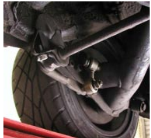
Figure 6: Complete type-2 sway bar setup on early car with no original sway bar option
