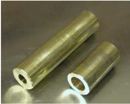
Figure 3: Original guide blank on the left; Modified bushing on the right
