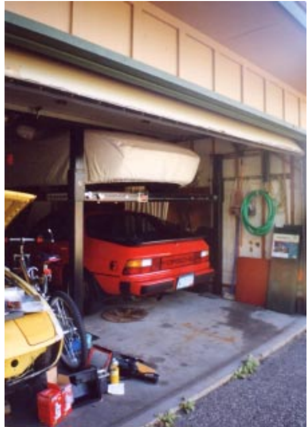
Mitch's garage showing car lift that has 1" tolerance at ceiling (photo courtesy of Mitch Berry)
