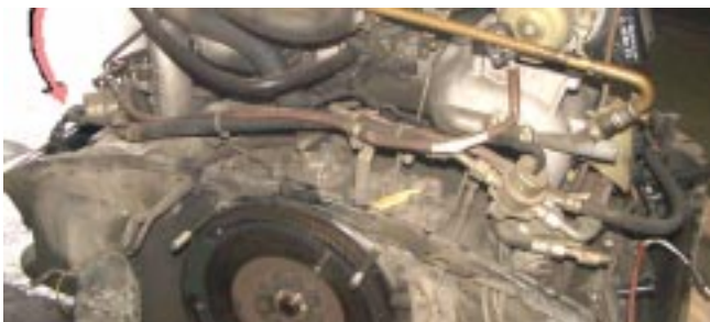
The failure point is usually the small black curved hose that connects at the fuel regulator (see arrow), photo by Steve Grosekemper
